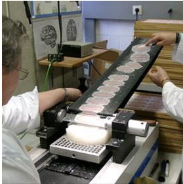
Figure 2. Researchers used a tool called a microtome to cut a brain into slices 20 micrometers thick (Image courtesy of Amunts, Zilles, Evans, et al.), (Nature News Whole human brain mapped in 3D, 2013).
